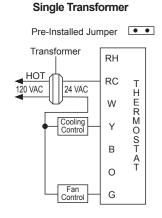
\*\* Note: Millivolt system may require a transformer and/or an isolation relay to operate properly
